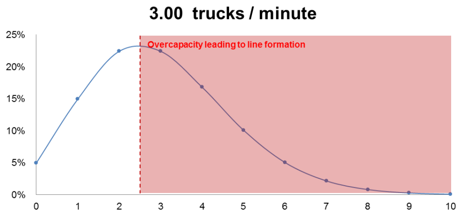
Figure 39. Poisson distribution considering an average arrival of 3.00 trucks / minute Source: Elaborated by the author
